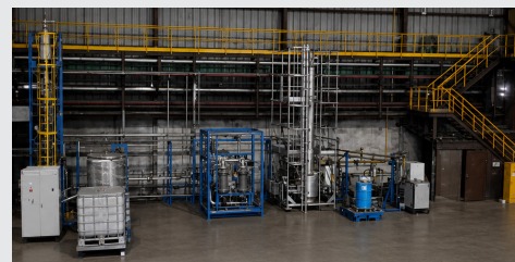
LLT CO 2 capture demonstrator with a capacity of 50 kg/h. © LLT.
