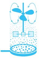
INCORPORATE AIR BUBBLES INTO THE CULTURE MEDIUM HOMOGENIZE THE PRODUCT IN THE TANK FLEXIBILITY, EFFICIENCY, RELIABILITY :
